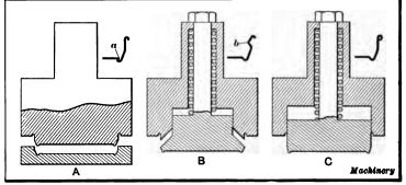
Fig. 17. Three Forms of Wiring Dies
